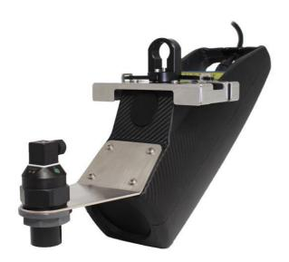
The RAVEN-EYE® is the newest non-contact RADAR area/velocity flow meter for open channel flow measurements from FLOW-TRONIC. The new sensor combines advanced digital Doppler radar velocity sensing technology with most modern and powerful DSP processor technology allowing a patent pending self-learning average velocity calculation. The need for empirical models or time consuming site calibration become obsolete.
